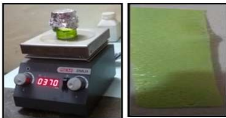
Figure 4: (a) Developed Zn-CuO-PMMA for 2:5 ratio solution (b) Zn-CuO of 2:5 doped PMMA Polymer Composite Film
