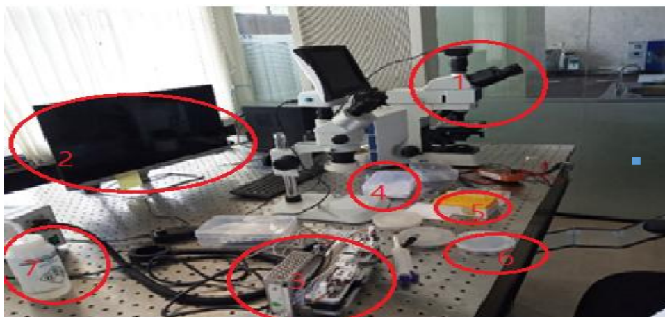
Figure 5: Characterization (a)V-I Characteristics of the micro cantilever (b) Experimental setup 1-Microscope, 2- GUI, 3-4-5-Purchased Antibodies, 6-Cleaner
