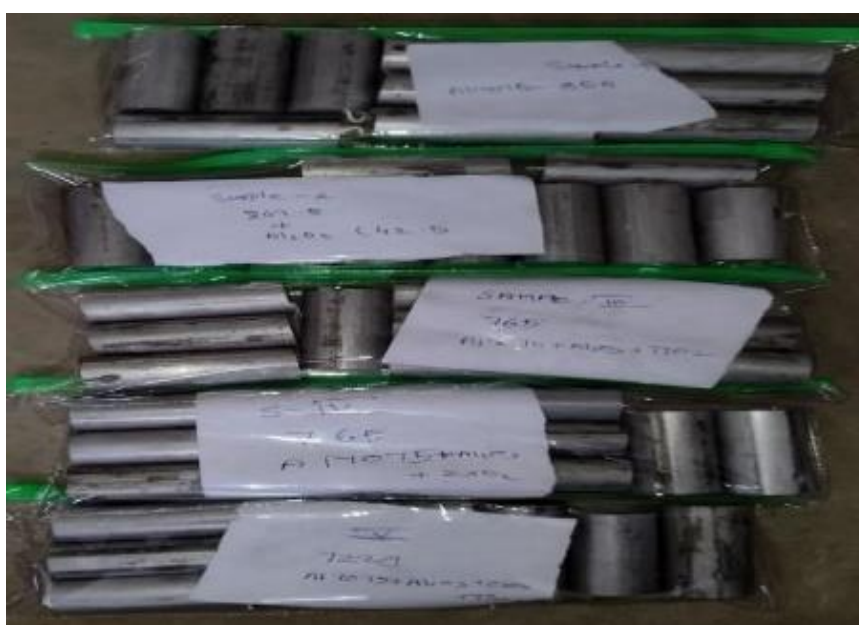
Figure 3: Before the casting process the rod is separated by weight percentages
