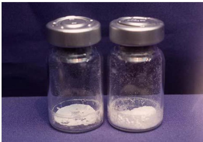
Figure 10: Collapsed Product – Critical Temperature was exceeded
