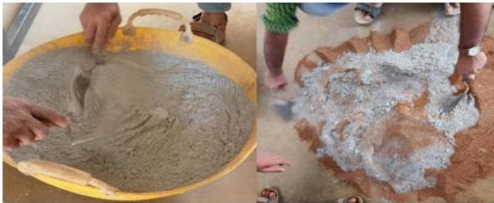
Figure 8: Blending AHA and lime
