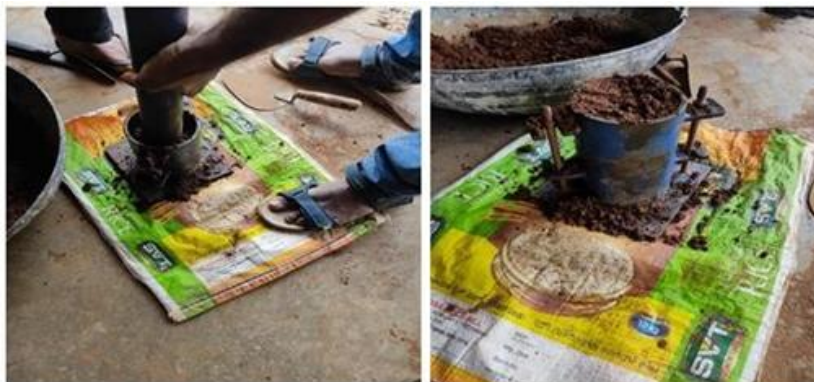
Figure 13: Standard Proctor Test
