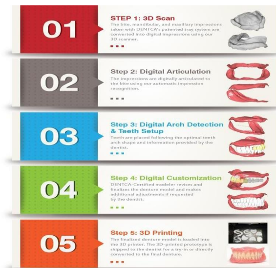
Figure 1: Steps in Fabrication of CAD/CAM Denture.
