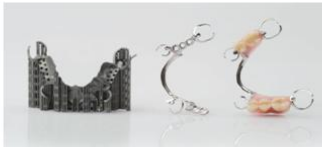
Figure 37: Laser sintered Removable Partial Denture
