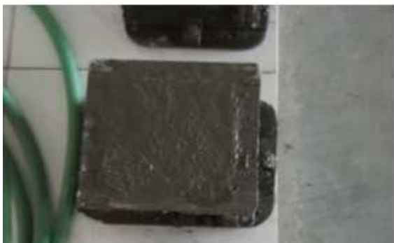
Figure 10: Added mixture in to the mould
