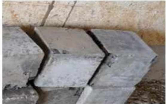
Figure 11: Demoulding of Blocks
