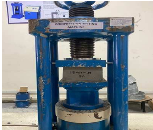
Figure 3: Compressive Strength Test of Cube
