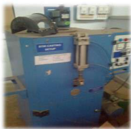
Figure 2: Stir Casting Furnace and Die
