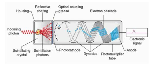
• This output light can be used as a measure of adsorbed radiation on scintillation detector. This emitted light when enters into photo-multiplier tube; it multiplies and amplifies even a small signal. So it becomes possible to measure alpha, beta or gamma radiation by scintillation detector.
