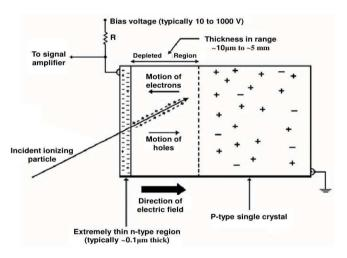
6. Solid State Detectors: They have high resolution, compactness and easy interpretation of output signal.
