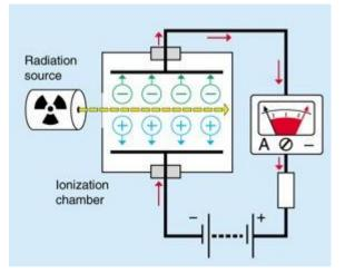
It comprises of a chamber filled with gas such as Argon, Helium, or Air, among others. The ionization chamber is outfitted with two electrodes maintained at varying electric potentials (50-100V for each cm of distance between two electrodes) and a measurement device to detect current flow. Radiation causes the ionization of gas molecules or ions, which results in the release of electrons, which displays changes in electric current.
