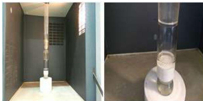
Figure 11(b): Microwave reactor and reactor vessel to accommodate HM catalyst.
