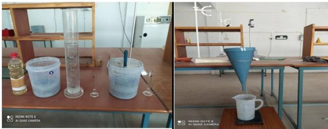
Figure 1: Cement, PCE, SMF, Marshcone Setup
