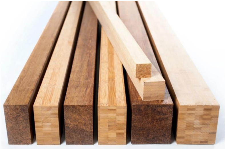
Figure 5: Bamboo composites (courtesy: Moso Studio).
