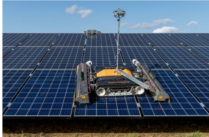
Figure 7: Automatic Wiper Based Cleaning
