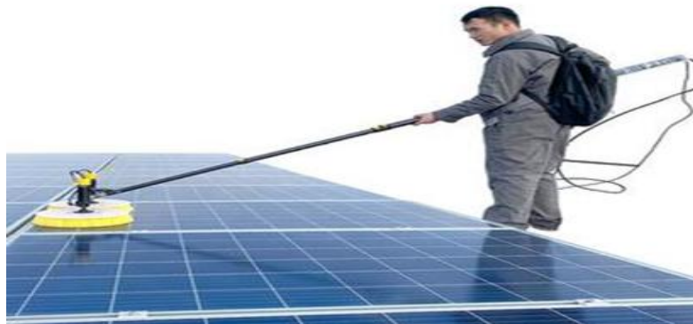
Figure 6: Vacuum Suction Cleaning
