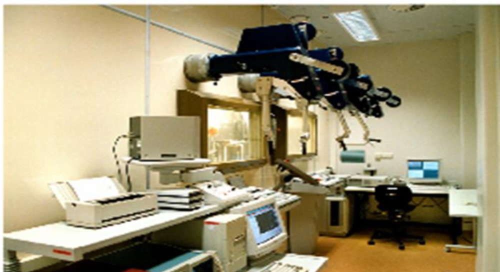
Figure 9: Hot cells with manipulators used for radioisotopes/radiopharmaceuticals production are available from commercial sources. [21]
