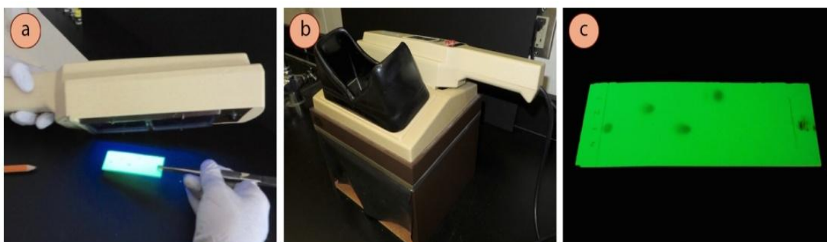
Figure 4: a) Tilting a UV lamp to visualize a TLC plate, b) Box to protect eyes from UV damage, c) Appearance under UV (Lisa Nichols, Butte College 2023).
