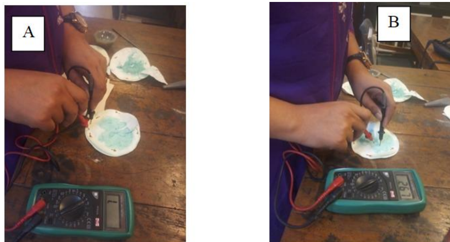
Figure 7: Electrical Conduction Seen Using Digital Multimeter for Two Cases (A) When There Is No Film) (B) At The Surface Of The Copper Film
