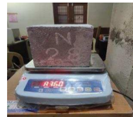
Figure. 4 : Weight of Cube After 28days Curing Normal
