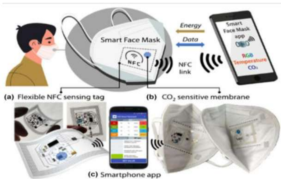
Figure 8: Schematic representation IoNT driven Smart Face Masks
