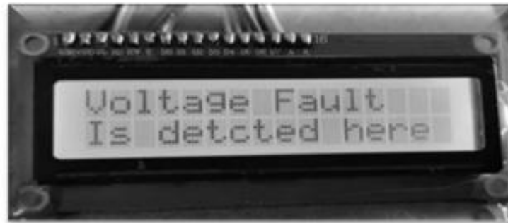
Figure 8: During Voltage Fault
