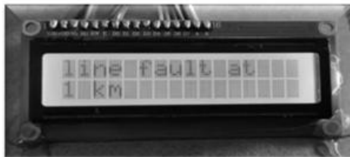
Figure 9: Line Fault at 1 km
