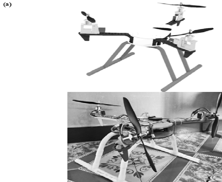
Figure 1. (a). CAD model (Isometric View) of Aerogi; (b). Real image of Aerogi
