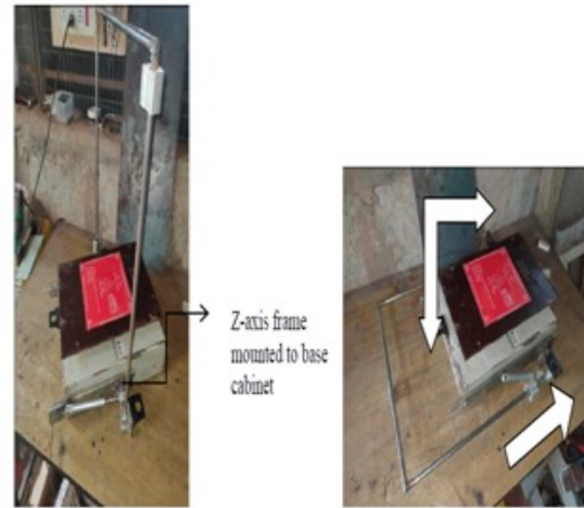
Figure 7: Folding of the Frame-Y Axis Frame and Carriage
