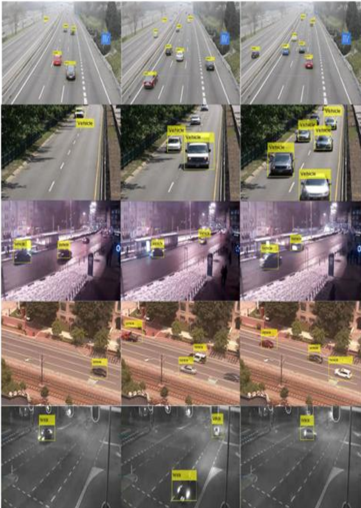
Figure 6: Detection of Vehicles on the Road from Different Camera Views By Day Scenes and Night Scenes
