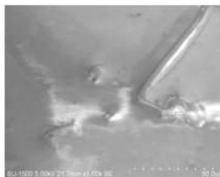
Figure 4.3b: SEM images of Fe 2 O 3 /PS at 50 μm
