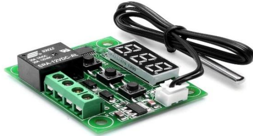
Figure 6: W1209 Temperature Control Switch
