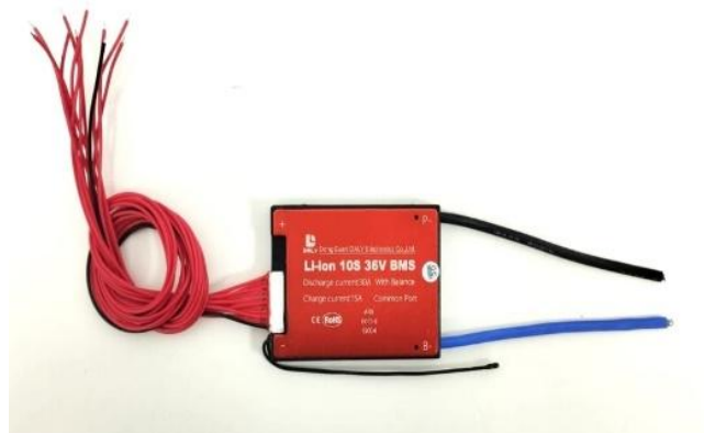
Figure 3: Battery Management System
