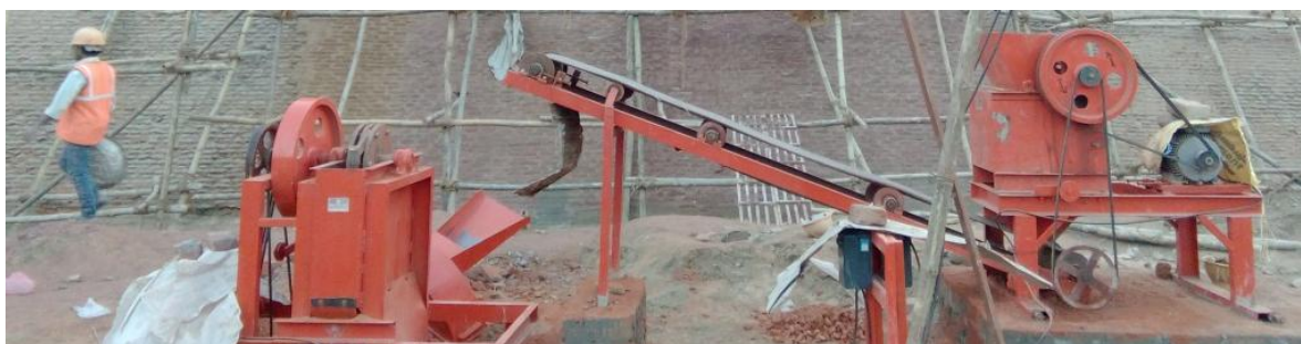
Figure 4: Showing Grinding Machine process of making Surkhi
