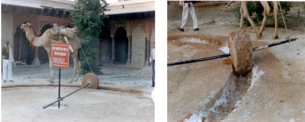
Figure 5: Showing Traditional lime mortar mill operated by camel
