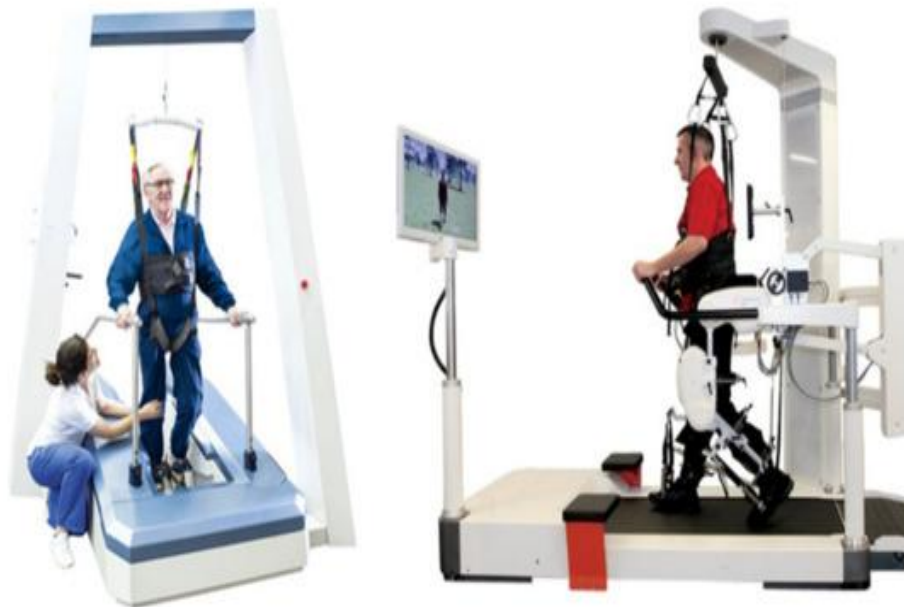
Figure 3. Robot-assisted gait trainer. Lyra (Thera Trainer, Hochdorf, Germany) (left); Lokomat (Hocoma, Volketswil, Switzerland) (right). Schicketmueller, A.; Lamprecht, J.; Hofmann, M.; Sailer, M.; Rose, G. Gait Event Detection for Stroke Patients during Robot-Assisted Gait Training. Sensors 2020, 20, 3399. https://doi.org/10.3390/s20123399
