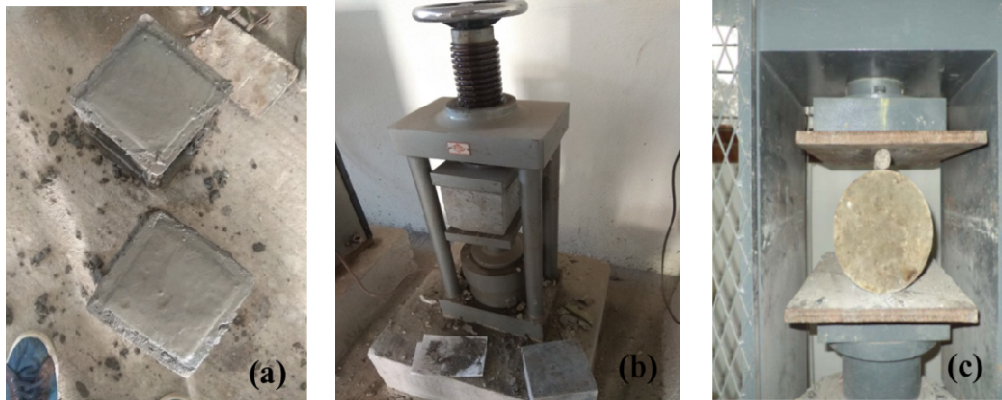
Figure 2: Experimental Setup (a. Casting b. Compressive Strength Setup c. Split Tensile Strength Setup)
