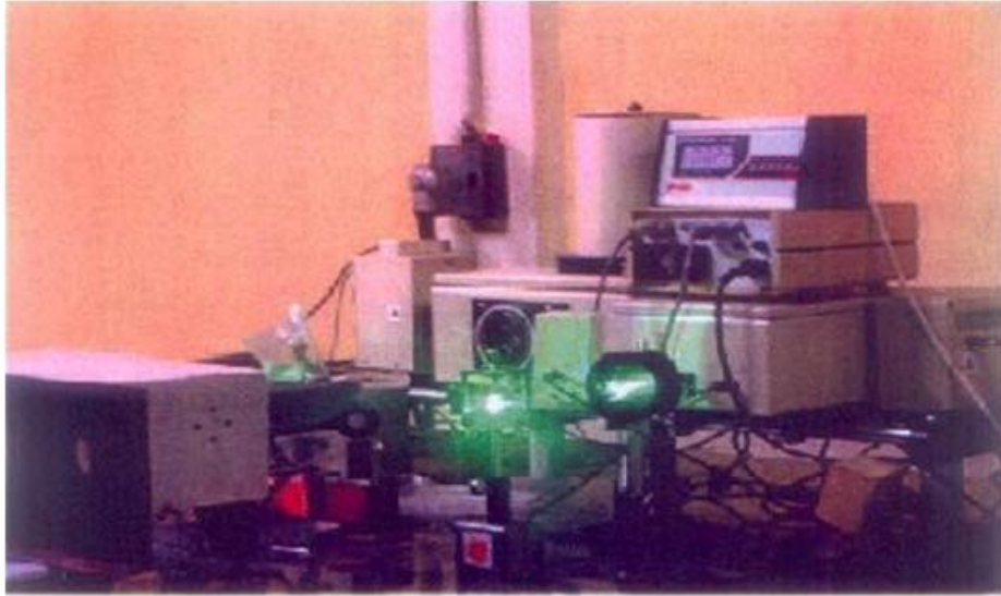
Figure 23: Experimental Set Up of Powder NLO Test
