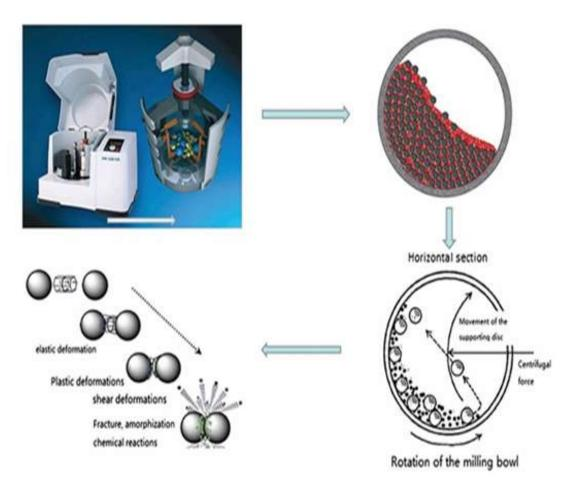
The ball milling method's basic idea. Reprinted from ref. 25 with permission. John Wiley & Sons, Ltd., 2016-2017.
