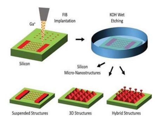
An illustration showing how bulk Si structuring with an ion beam can be used to create 3D micro-nanostructures. This involves anisotropic wet etching in KOH solution, anisotropic implantation in Si using Ga FIB lithography, mask writing at nanometer resolution, and fabrication of Si micro-nanostructures by selectively removing the unimplanted region.
