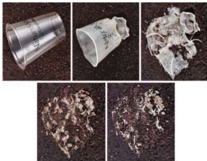
Figure 2: Biodegradation of a Disposable Cup Made from PLA. Time Sequence: 1, 15 and 30 Days (top); 45 and 58 Days (bottom) [2]
