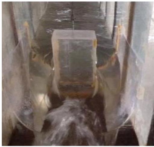
Figure 4: Installed Circular Contracted Flume inside the Hydraulic Flume in Working Condition
