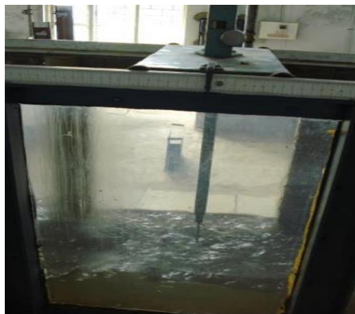
Figure 5: Point Gauge Used to Record Profiles of Water Surfaces
