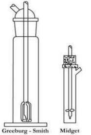
**11. Two types of impingers:** Initial research suggests that the impinger is marginally less effective than the fritted absorber when it comes to gathering gaseous pollutants. Under ideal operating conditions, the fritted-glass absorber was observed to outperform midget
