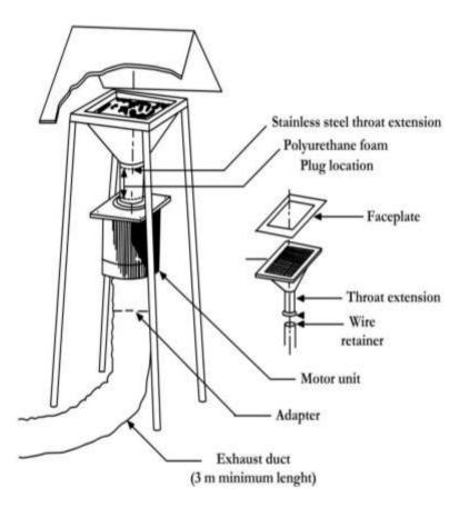
6. Assembled sampler and shelter with exploded view of the filter holder
