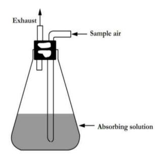
7. Absorption device adapted from an Erlenmeyer flash: Gas enters the absorbent solution through the uncontrolled aperture. These absorbers come in a range of varieties. They are often made of glass and might have a cylindrical or conical shape. The several devices have typical flow rates ranging from 1 to 5 liters per minute. Two types of absorbers are commonly utilized in atmospheric sampling: (a) fritted-glass absorbers, also known as bubblers, and (b) impingers.
