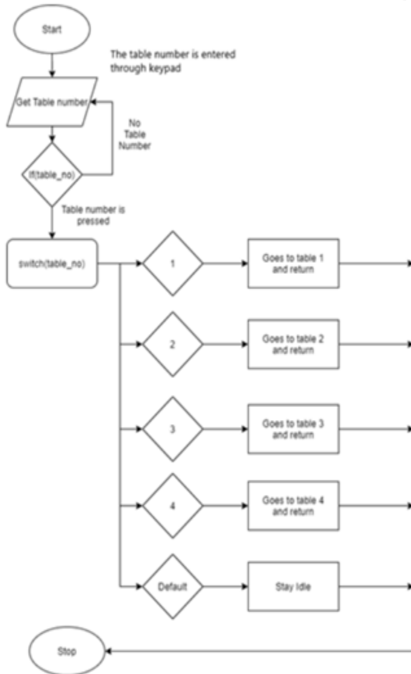
Figure 7: Flow chart of basic ideology of working
