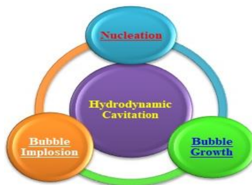
Figure 2: Pictorial representation of HC Mechanism
