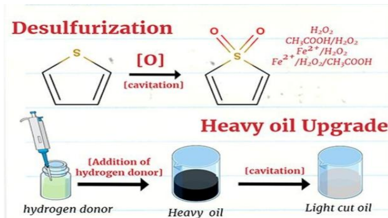
Figure 6: Desulfurization methodology by HC[8]
