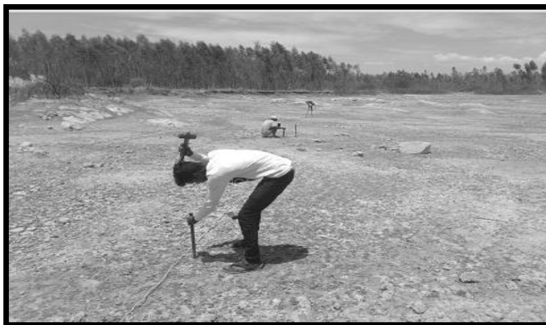
Figure 3: Field Work Data Collection and Electrode Layout
