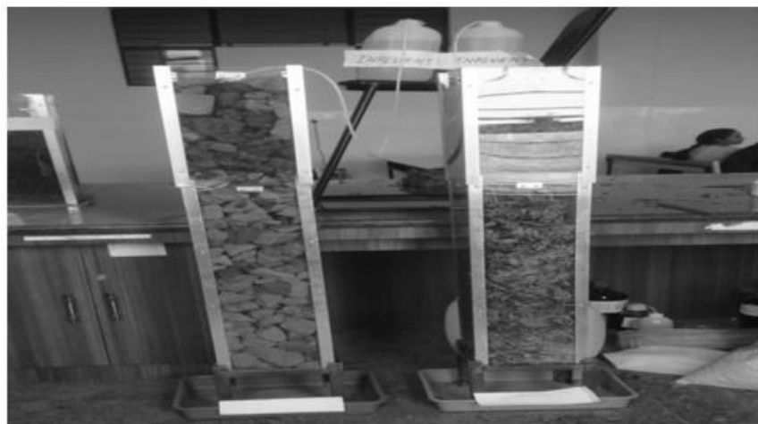
Figure 4: Setup 3 Where Materials Filled to a Height of 1.5m in the Treatment Unit
