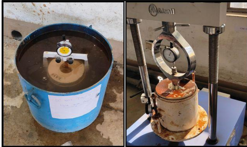
Figure 1: Soaked CBR Test setup.
