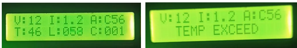
Figure 9 (d): Temp Limit Exceed Cleaning Process
