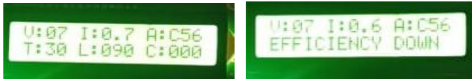
Figure 9 (b): Low efficiency Cleaning Process
