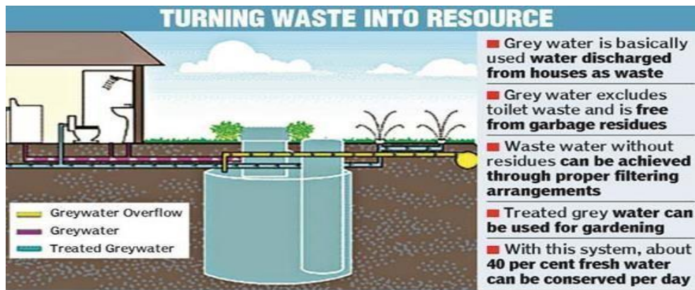
Figure 2: Grey water purification [32]
