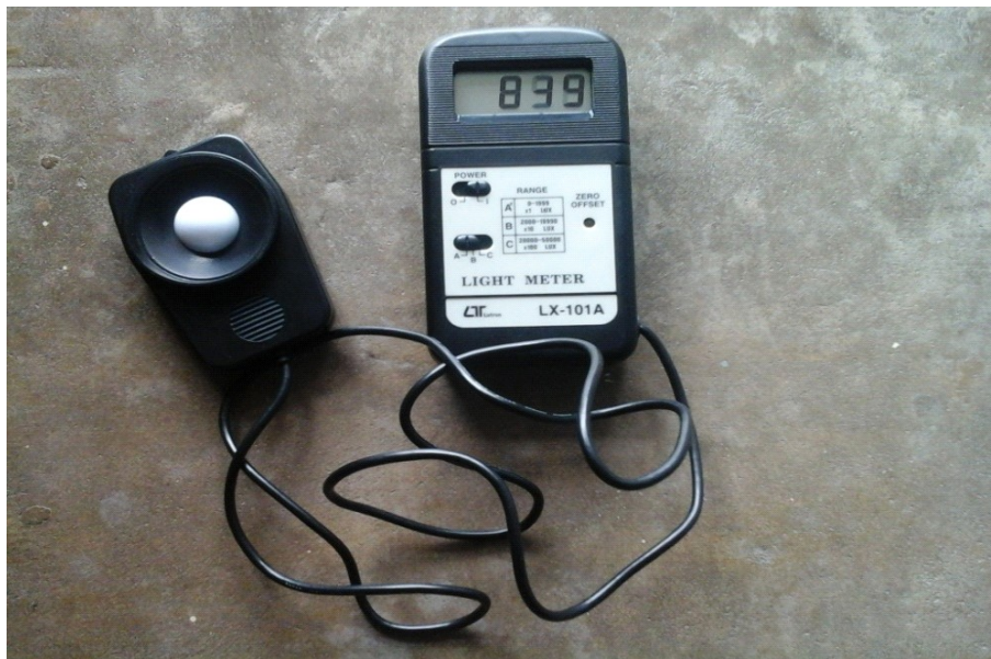
Plate 4 : Lux meter (Lux Meter LX-101A) used for light intensity study of Bir Bikram Memorial College buildings
