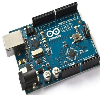
Figure 2: Arduino Uno R3
