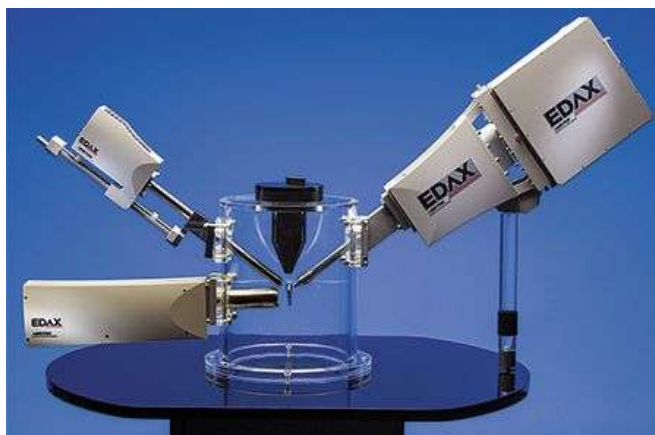
Figure 18: Instrumental set up of EDAX
