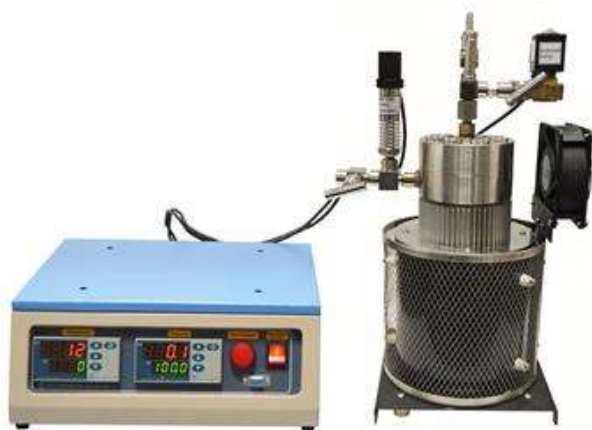
Figure 4: Instrumental set up of hydrothermal/ solvothermal method
