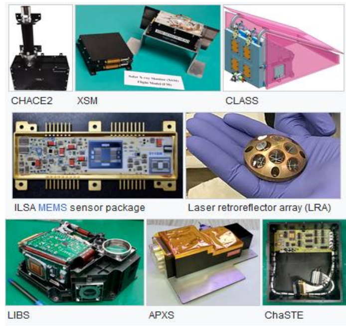
Figure 12: Pragyan Rover Instruments
