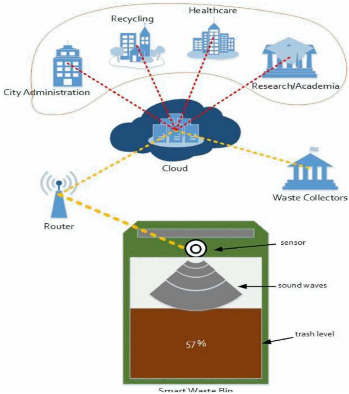
Figure 2: Cloud-based smart waste management architecture (Aazam et al., 2016)
