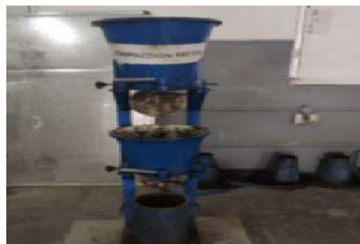
Figure 5: Compaction Factor Test
