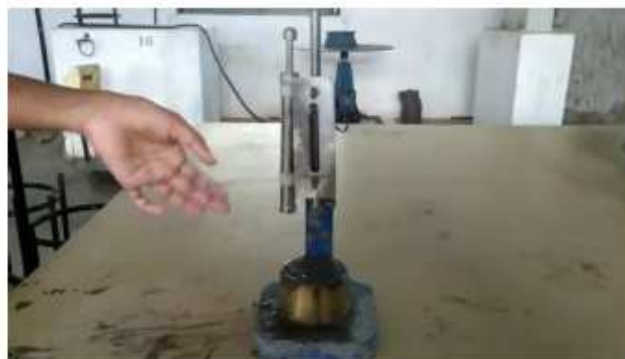
Figure 1: Setting Time of Cement
