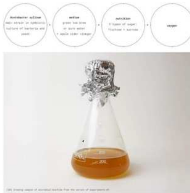
Figure 4 : Growth Medium for the Synthesis of Bacterial Cellulose (source : Feasibility Of Bacterial Cellulose In Furniture Design, bachelor's thesis, Monika Faidi 2017)
