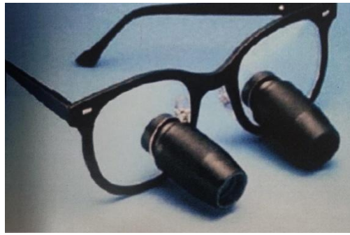
Figure 7: Keplerian System of Loupes
