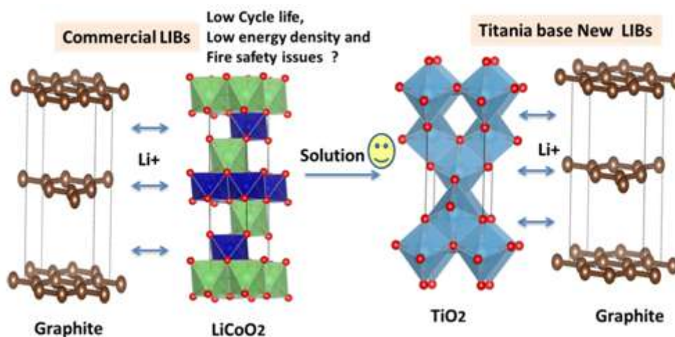
Figure 5: Titania based nanostructures as electrodes in lithium ion batteries
