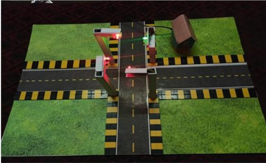
Figure 6: Four Way Traffic Control System
